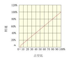
When the duty ratio is 4%, the motor speed is 4% of the maximum speed; when the duty ratio is 100%, the speed of the motor is the maximum value. The maximum speed value depends on the motor size and supply voltage.
