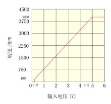
When the input voltage is about 0.2V, the motor speed is 160rpm; when the input voltage is about 5V, the speed of the motor is 4000rpm.
