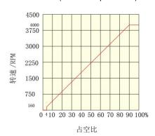
When the duty ratio is 4%, the motor speed is 160 rpm; when the duty ratio is 100%, the speed of the motor is the highest speed, 4000 rpm.
